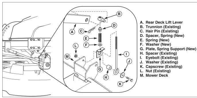
Figure 1. Counter Balance Installation
